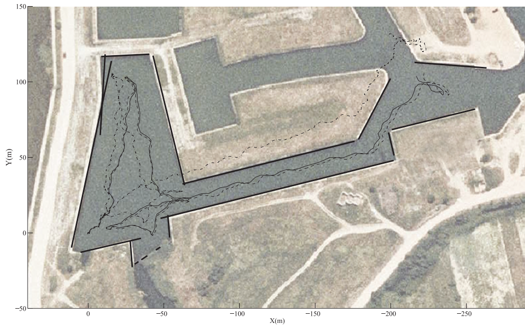
Figure 6.17: The resulting global map together with the dead-reckoning (dash-dotted line), GPS (dashed line) and SLAM (solid line) trajectories represented over a satellite image of the scenario.
