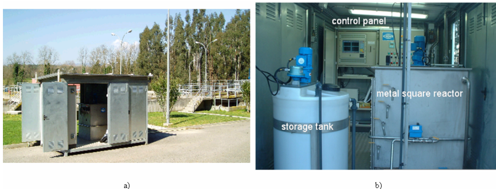
Figure 2.3: a) Semi-industrial Pilot Plant b) Operational Schema of the semi-industrial pilot plant SBR
