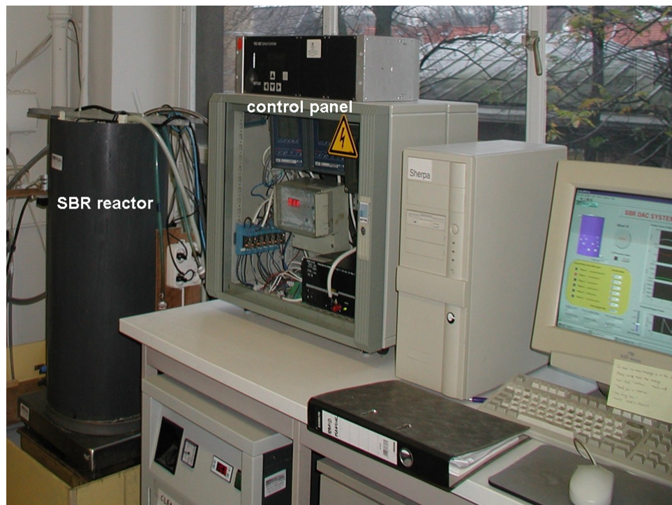
Figure 2.11: Lab-scale plant from BIOMATH
