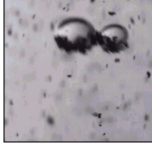
Figure 3.26: Frame corresponding to the video july21_susp_shp_120_200_sulf_1fast, two bubbles were held together by ink particles.
