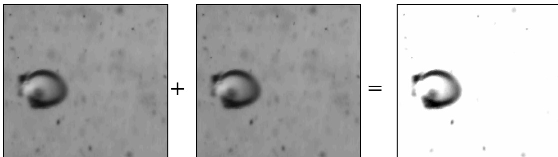
Figure 3.23: Result of applying addition operation to an image.
