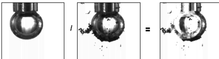
Figure 3.6: Results of combining two images with division operation. During ink injection a needle displacement has occurred.
