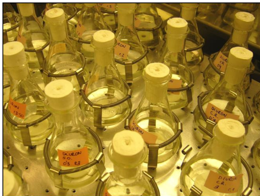
Fig. 7 Algal cultures of Scenedesmus obliquus exposed to the phenylurea herbicide diuron during the mixture experiment.
