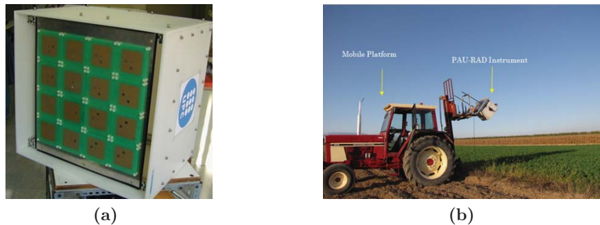
Figure 2.2. PAU-RAD instrument a) without radome, and b) measuring an alfalfa field, in the 2010 Palau d'Anglesola field campaign.
