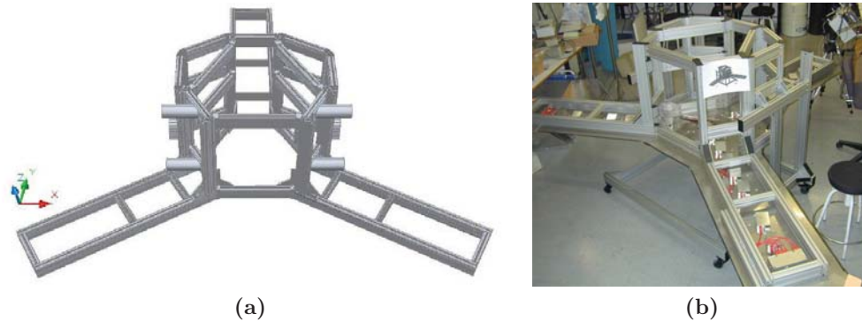
Figure 7.77. a) 3D scheme of PAU-SA's chassis (reinforced version), and b) Picture of PAU-SA's chassis (reinforced version) located in the D3-213 laboratory.
