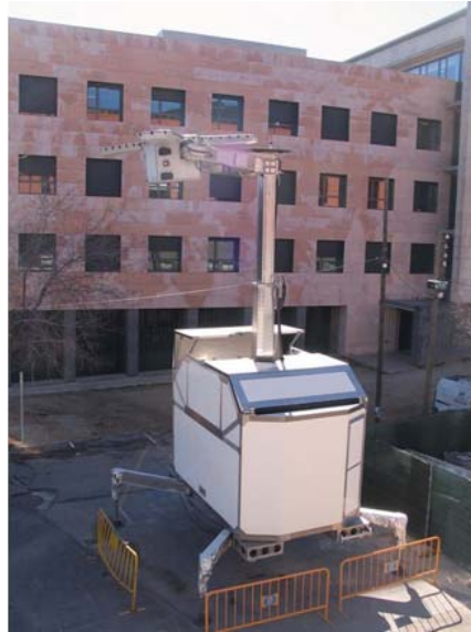
Figure 5.16. PAU-SA instrument pointing to the zenith for absolute amplitude calibration and GPS satellites imaging.
