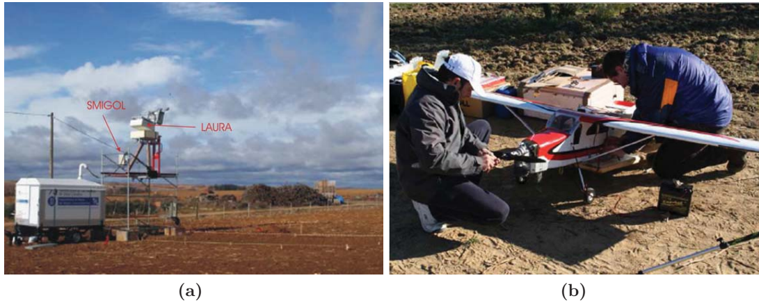
Figure 2.11. GRAJO field campaign: a) L-Band AUTomatic Radiometer (LAURA) and SMIGOL deployed instruments [53], and b) preparing the UAV of PAU-ORA for measuring [54].
