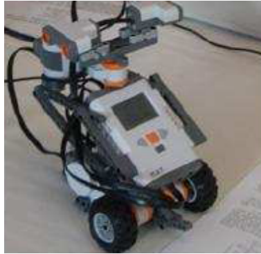
Figure 4.1: Robot LEGO Mindstorms NXT.
