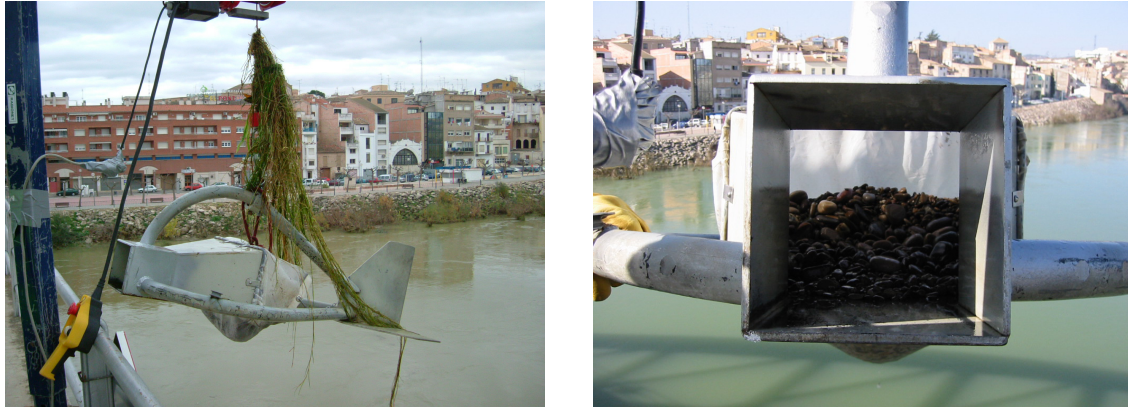
Figure 4. Helley-Smith bedload sampler 152-mm intake
