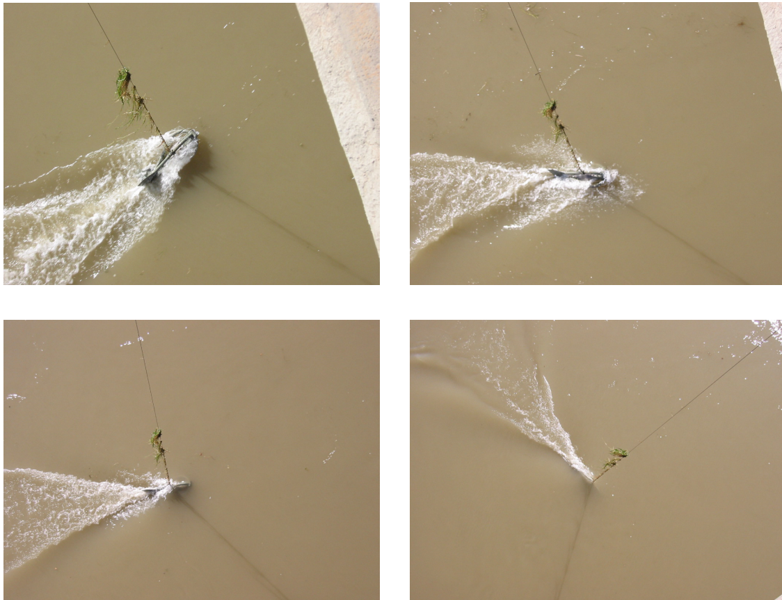
Figure 5. Deployment of a 76-mm intake Helley-Smith 76-mm sampler during February 5 th 2003 at the Móra d'Ebre Bridge Monitoring Section
