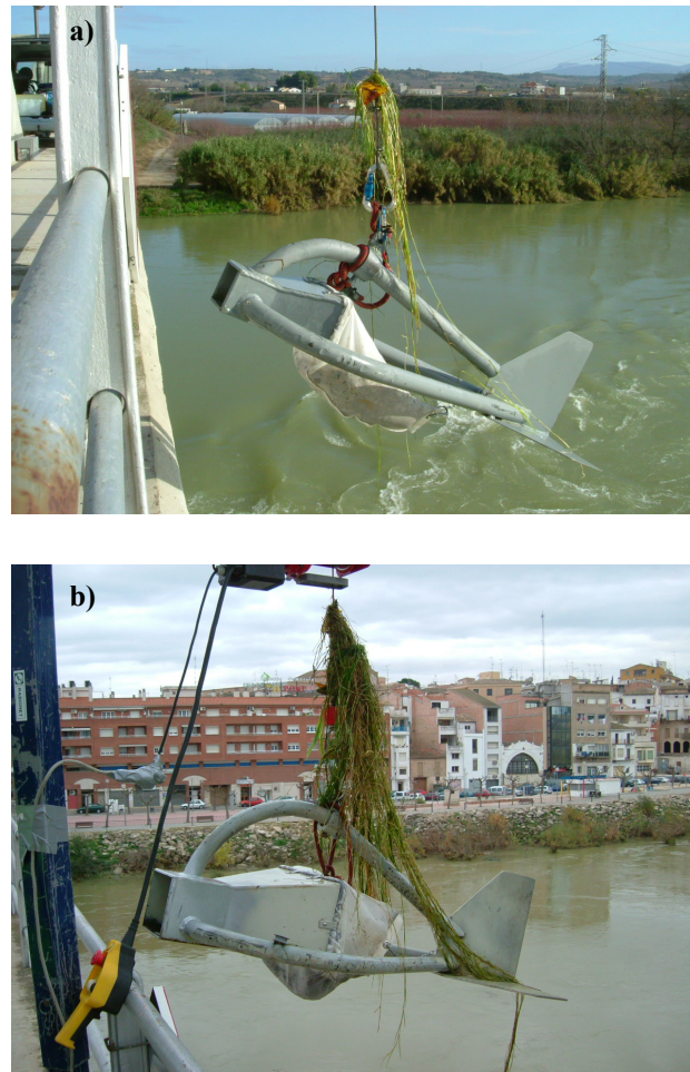
Figure 3 (C2P1). (a) Cable suspended Helley-Smith sampler 76-mm intake and (b) cable suspended Helley-Smith sampler 152-mm intake at the Móra d'Ebre Monitoring Section
