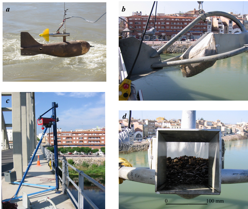
Figure 2 (C3P1). Field equipment to measure discharge and sediment transport from bridges: a) OTT C31 current metre attached to a cable suspended US DH74 sediment sampler, b) cable suspended 76 kg Helley Smith Sampler, c) automatic crane for suspension of sampling equipment, and d) intake (152 mm) of the Helley Smith Sampler, showing bedload material captured on February 11 th 2003. Photos by the authors (February 2003)
