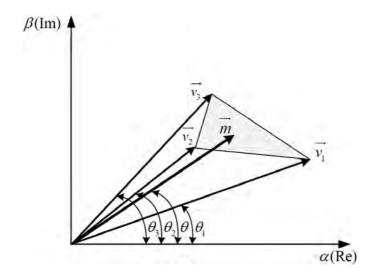
Figure 5.9: Limiting area to generate the reference vector by using the triangle connecting of three vectors
