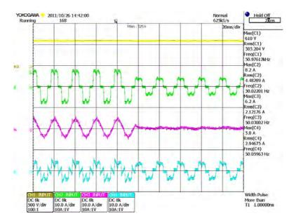
Figure 8.13: dc-bus voltage, load, grid, and DG currents before and after remove of additional load from the grid
