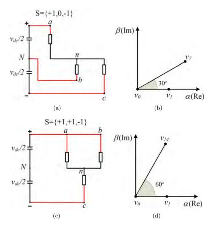
Figure 5.8: Generation of middle and external voltage vectors according to the switching states
