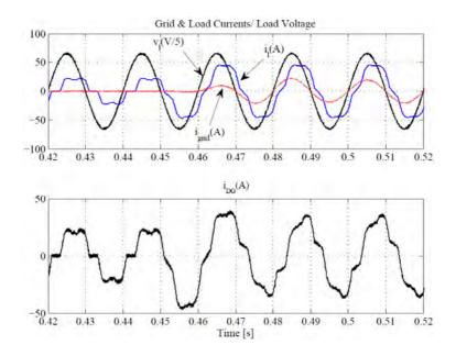
Figure 7.18: Grid current, load voltage and load current before and after connection of additional RL loads to the grid
