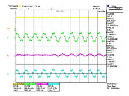
Figure 8.16: dc-bus voltage, load, grid, and DG currents before and after linear load increment
