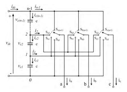
Figure 3.3: Schematic diagram of the n-level diode-clamped converter
