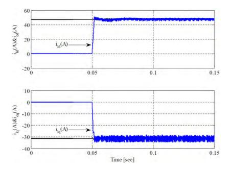
Figure 6.5: Reference and injected currents according to the dynamic performance of the controller
