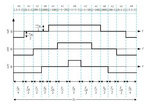
Figure 5.18: Sequence of voltage vectors for the first region of sector (I)
