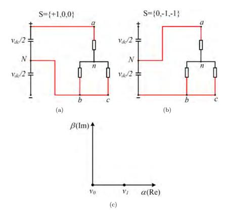
Figure 5.7: Generation of internal voltage vectors according to the switching states
