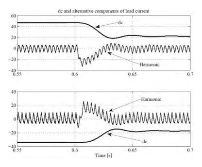
Figure 7.23: d and q-components of load currents before and after disconnection of additional RL load from the grid
