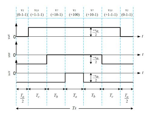
Figure 5.19: Sequence of voltage vectors for the second region of sector (I)
