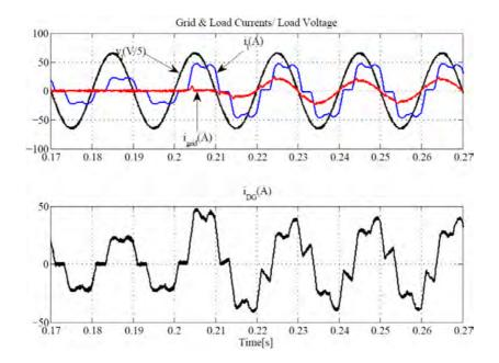
Figure 7.3: Grid, load, DG currents and load voltage before and after connection of additional load
