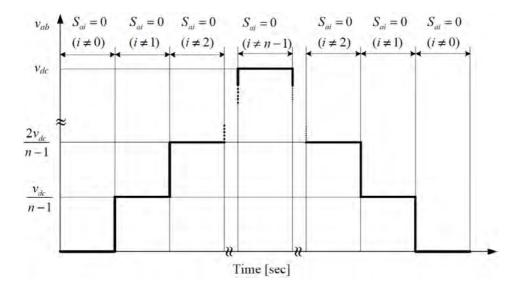
Figure 3.4: Line voltage waveform for an n-level diode-clamped converter
