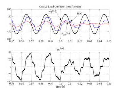
Figure 7.19: Grid current, load voltage and load current before and after disconnection of additional RL loads to the grid
