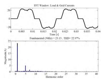
Figure 7.8: Load current spectra before connection of DG link to the grid
