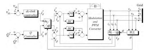
Figure 4.3: General schematic diagram for  $\alpha\beta$  frame control strategy
