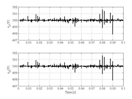
Figure 5.21: Voltage of dc capacitors in a NPC converter
