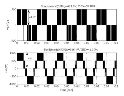
Figure 5.22: Phase and line voltages of NPC converter
