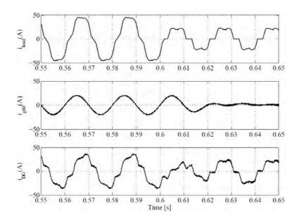
Figure 7.22: Load current, non-linear link current and grid current before and after disconnection of additional RL load
