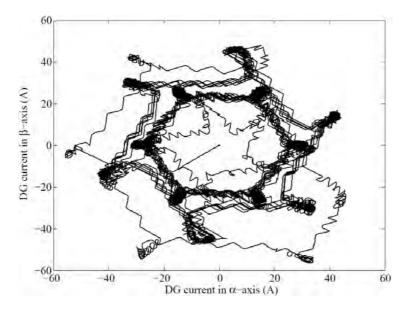
Figure 7.13: Trajectory of DG currents during connection of additional load to the grid in  $\alpha\beta$  representation
