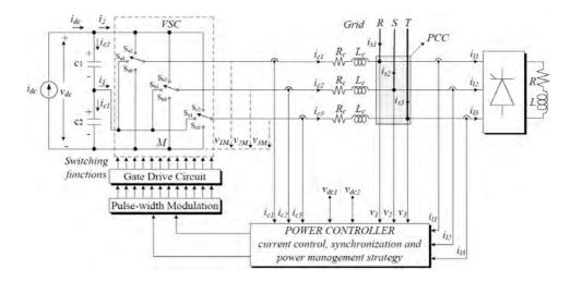
Figure 2.2: Schematic diagram and control functions of DG system based on three-level VSC
