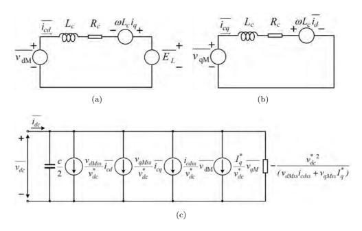
Figure 4.7: Equivalent small-signal circuit
