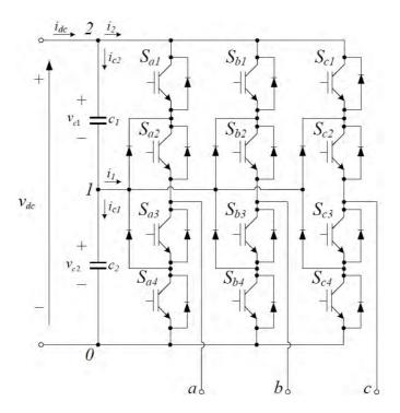
Figure 3.1: Three-level NPC converter
