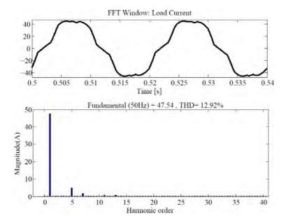
Figure 7.20: Load current spectra after connection of additional RL load to the grid
