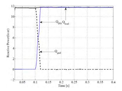
Figure 7.35: Grid, load and DG link reactive power, before and after integration of DG resources to the grid, and compensation of unbalanced load
