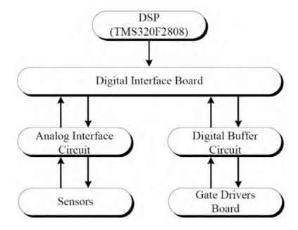
Figure 8.5: Architecture of the Sussie digital controller board
