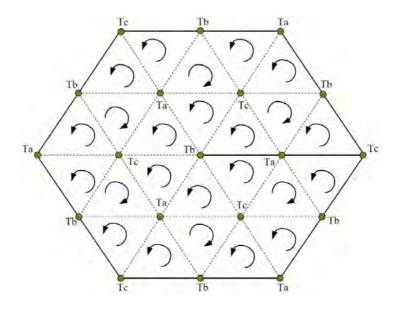
Figure 5.17: Switching sequence for three-level converter
