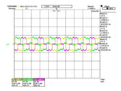
Figure 8.9: Load and grid current before connection of DG to the grid
