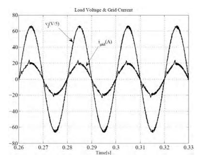
Figure 7.5: Phase-to-neutral voltage and grid current for phase (a)
