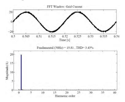
Figure 7.21: Grid current spectra after connection of additional RL load to the grid
