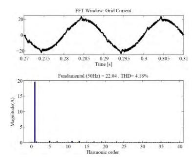
Figure 7.10: Grid current spectra after connection of additional load to the grid
