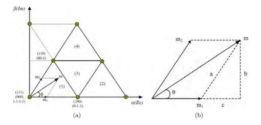
Figure 5.13: Projection of the normalized reference vector in the first sextant
