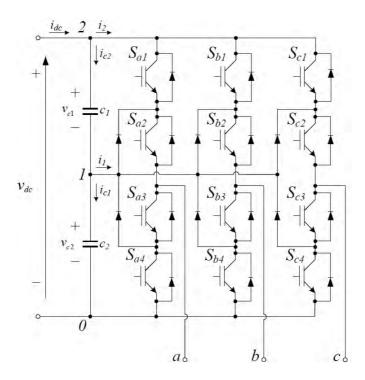
Figure 5.2: Schematic diagram of three-phase three-level diode-clamped converter
