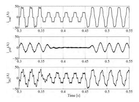
Figure 7.16: Load, grid and DG link currents before and after connection of additional RL load to the grid
