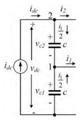
Figure 6.12: dc-side of proposed converter while NP current is not zero
