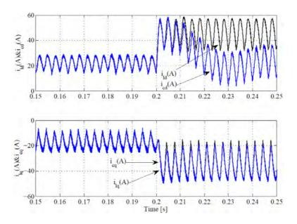
Figure 7.7: Reference currents track the load current after additional load increment
