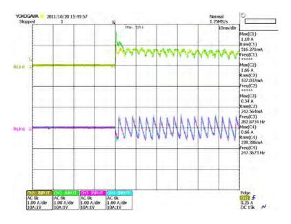
Figure 8.14: Reference currents track the load current after integration of DG to the grid
