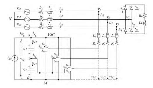
Figure 4.6: Proposed DG model based on three-level NPC converter
