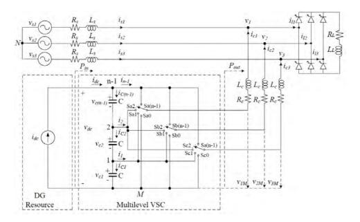
Figure 4.1: Schematic diagram of proposed DG model based on multilevel converter
