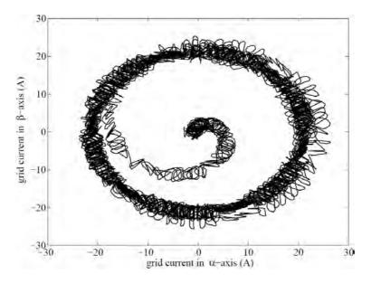
Figure 7.12: Trajectory of grid current after connection of additional load to the grid in  $\alpha\beta$  representation
