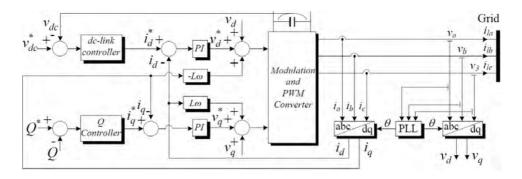
Figure 4.2: General schematic diagram for dq control structure
