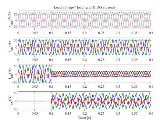
Figure 7.30: Load voltage, load, grid, and DG currents before and after connection of DG link into ac grid for compensation of non-linear unbalanced load
