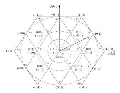
Figure 5.4: Space Vectors states for three-level NPC converter
