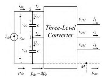
Figure 6.10: Voltage and current components in NPC converter
