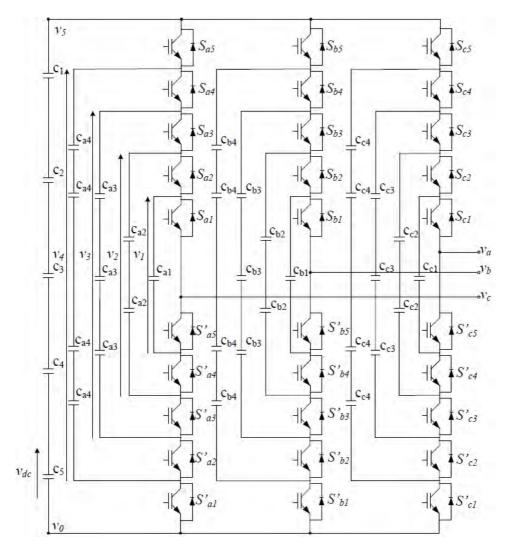
Figure 3.5: Schematic diagram of a six-level flying capacitor converter
