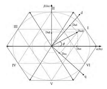
Figure 6.13: Voltage space phasors and related switching states
