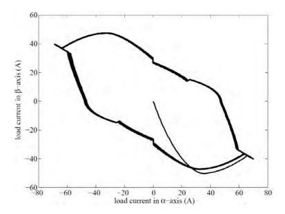
Figure 7.31: Trajectory of the unbalanced load current in  $\alpha\beta$  representation
