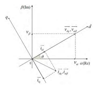
Figure 4.4: Voltage and current components in stationary and rotating synchronous reference frame
