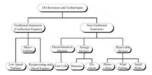
Figure 2.1: Different DG resources and technologies
