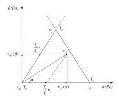
Figure 5.15: Switching times calculation for first region of sector (I)
