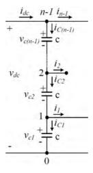
Figure 4.5: dc side of the proposed converter model
