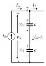
Figure 6.11: dc-side of interfaced converter while NP current is zero
