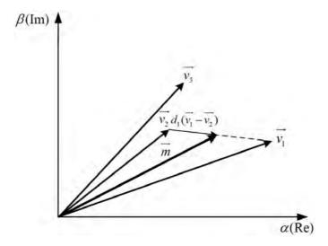
Figure 5.10: Boundary of the area, calculated by imposing zero value into the  $d_3$
