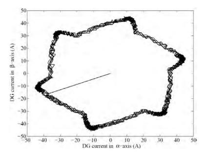
Figure 7.26: Trajectory of DG link current before and during connection of additional linear load to the grid in  $\alpha\beta$  representation
