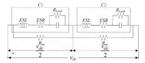
Figure 6.8: Equivalent circuit of capacitor with voltage sharing breeder resistance
