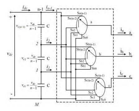
Figure 5.1: Schematic diagram of three-phase multilevel diode-clamped converter
