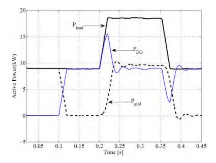
Figure 7.14: Grid, load and DG active power, during integration of DG resources to the grid, before and after connection and disconnection of additional load to the grid
