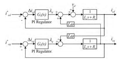
Figure 6.1: Complex vector block diagram of d and q-axis with a decoupling form of the synchronous frame PI current regulator
