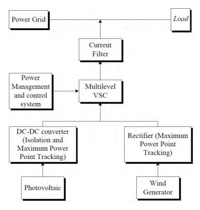
Figure 3.7: Power injection into the power grid by use of multilevel converter
