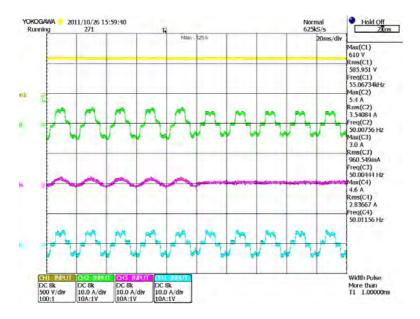
Figure 8.17: dc-bus voltage, load, grid, and DG currents before and after linear load increment
