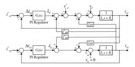
Figure 6.2: Control block diagram of d and q-axis current control loop
