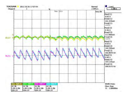
Figure 8.18: Reference currents track the load current before and after additional linear load increment
