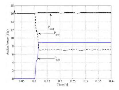
Figure 7.34: Grid, load and DG link active power, before and after integration of DG resources to the grid, and compensation of unbalanced load
