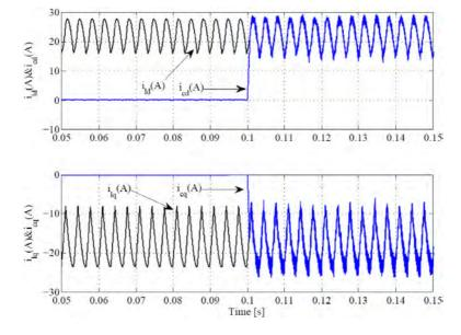
Figure 7.6: Reference currents track the load current after interconnection of DG resources to the grid
