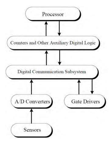
Figure 8.3: Structure of the digital controller for power electronics systems
