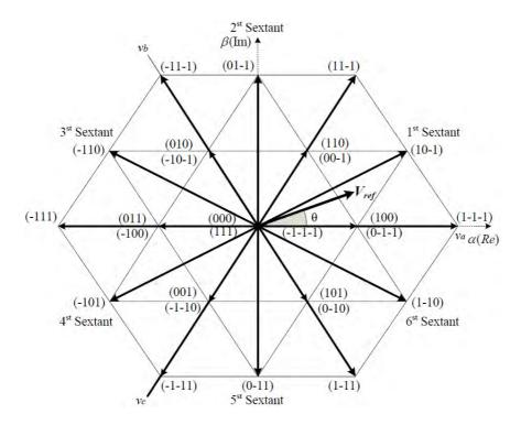
Figure 6.6: Space vector diagram of the three-level NPC converter
