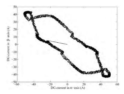
Figure 7.33: Trajectory of the DG current in  $\alpha\beta$  representation
