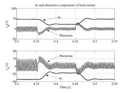
Figure 7.17: d and q- components of load currents before and after connection of additional RL load to the grid
