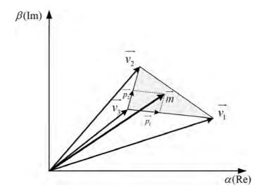
Figure 5.11: Projections of the reference vector  $\vec{m}$  ( $\vec{p_2}$  and  $\vec{p_1}$ )
