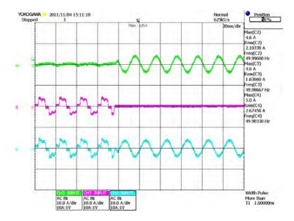
Figure 8.19: Steady-state operation of the DG link for injection of maximum available active power from DG source to the power grid, continuously
