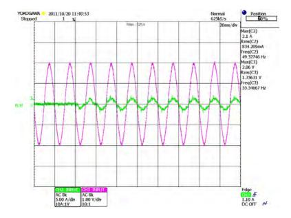
Figure 8.12: Phase-to-Phase voltage and grid current for phases (ab)
