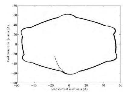
Figure 7.24: Trajectory of load current before and after connection of additional linear load to the grid in  $\alpha\beta$  representation
