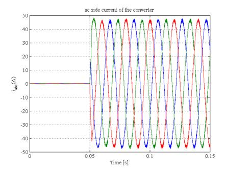
Figure 6.14: Evaluation of the ac side current of the interfaced converter in the abc reference frame
