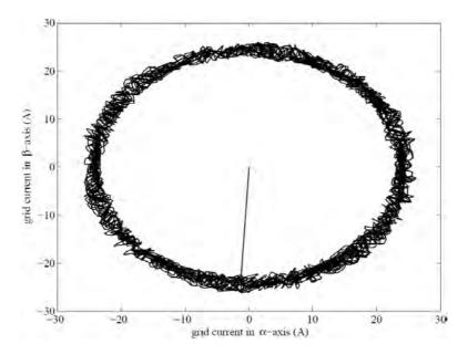
Figure 7.25: Trajectory of grid current before and during connection of additional linear load to the grid in  $\alpha\beta$  representation
