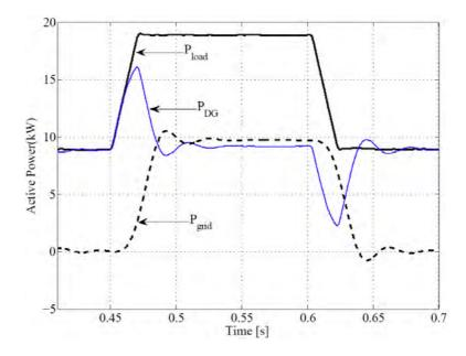
Figure 7.28: Grid, Load and DG link active power, during integration of DG resources to the grid, before and after connection and disconnection of additional non-linear and linear loads to the grid
