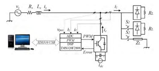
Figure 8.7: Experimental set-up of the proposed DG system
