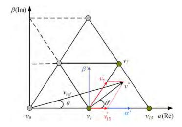
Figure 5.16: Switching times calculation for second region of sector (I)
