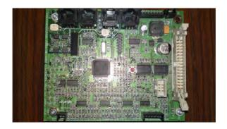
Figure 8.4: DSP based Power Electronics control board
