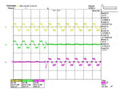
Figure 8.10: Load, grid, and DG currents before and after connection of DG link to the power grid
