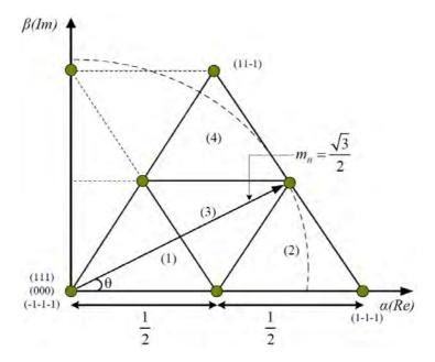
Figure 5.12: Maximum length of the normalized reference vector in steadystate condition
