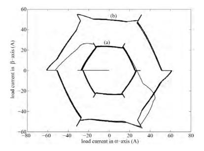
Figure 7.11: Trajectory of load current before and after connection of additional load to the grid in  $\alpha\beta$  representation
