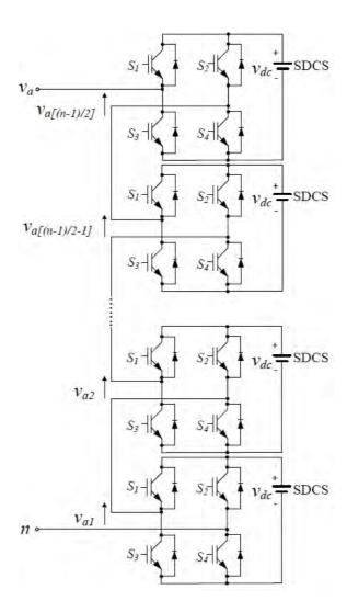
Figure 3.6: Single-phase schematic diagram of a multilevel cascaded H-bridges converter
