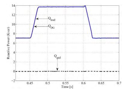
Figure 7.29: Grid, Load and DG link reactive power, during integration of DG resources to the grid, before and after connection and disconnection of additional non-linear and linear loads to the grid
