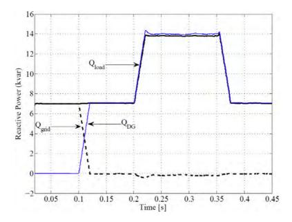
Figure 7.15: Grid, load and DG reactive power, during integration of DG resources to the grid, before and after connection and disconnection of additional load to the grid
