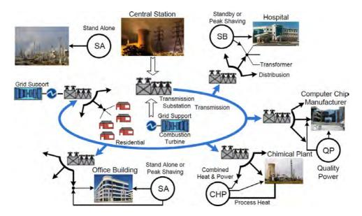
Figure 1.1: Summary of DG applications in electrical networks
