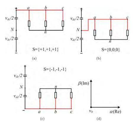
Figure 5.6: Generation of zero voltage vectors according to the switching states
