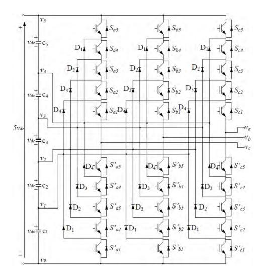
Figure 3.2: Schematic diagram of three-phase six-level diode-clamped converter
