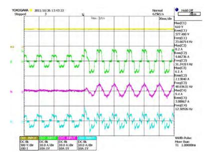
Figure 8.11: dc-bus voltage, load, grid, and DG currents before and after connection of additional load to the grid
