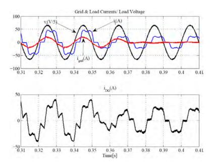
Figure 7.4: Grid, load, DG currents and load voltage before and after disconnection of additional load
