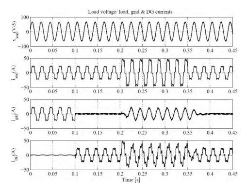
Figure 7.2: Load voltage, load, grid, and DG currents before and after connection of DG and before and after connection and disconnection of additional load to the grid
