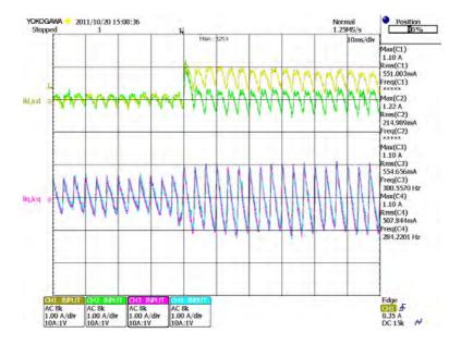
Figure 8.15: Reference currents track the load current after connection of additional load to the grid
