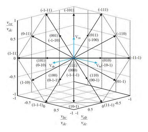
Figure 5.3: Switching states of a three-level converter
