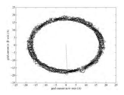
Figure 7.32: Trajectory of the grid current in  $\alpha\beta$  representation
