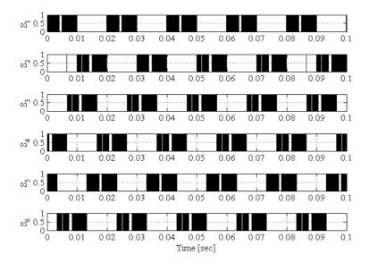
Figure 5.20: Switching state for six upper IGBTs in a NPC converter
