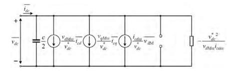
Figure 4.8: Equivalent small-signal circuit model for unity power factor
