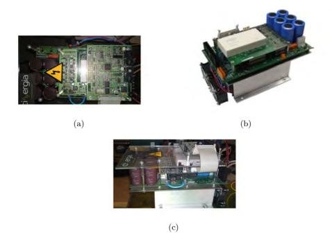
Figure 8.1: Experimental setup platform (a). Control, (b). Drive and power, (c). General structure
