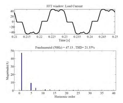
Figure 7.9: Load current spectra after connection of additional load to the grid
