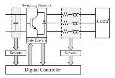
Figure 8.2: Power electronics system
