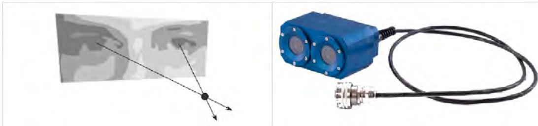
Figure 1.1: Comparison between human stereo-vision and a classical passive stereo-vision device.
