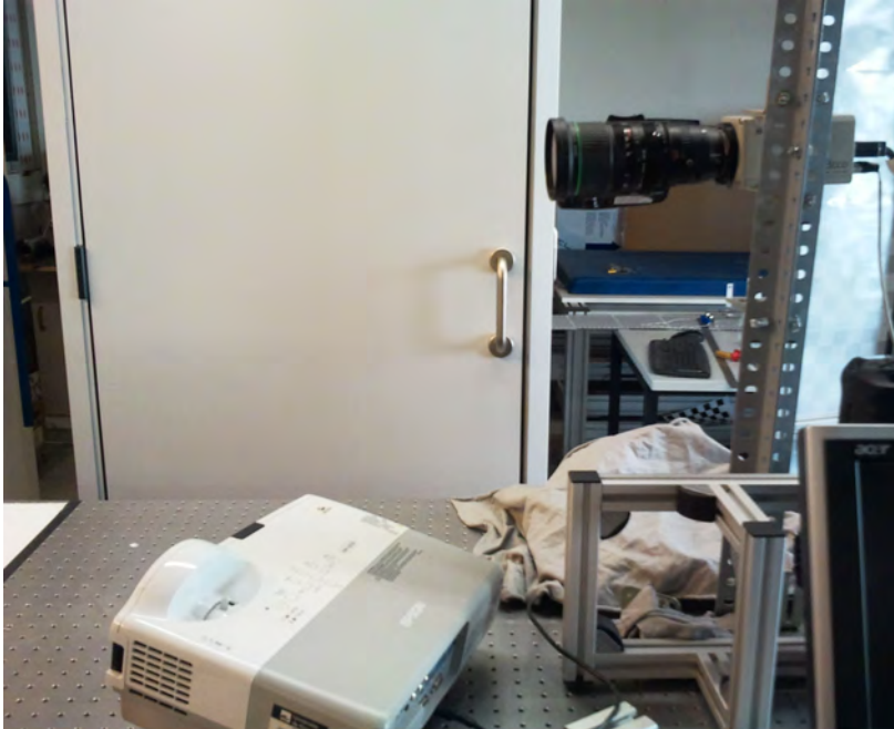
Figure A.6: Projector-camera setup used to test the proposed algorithm.
