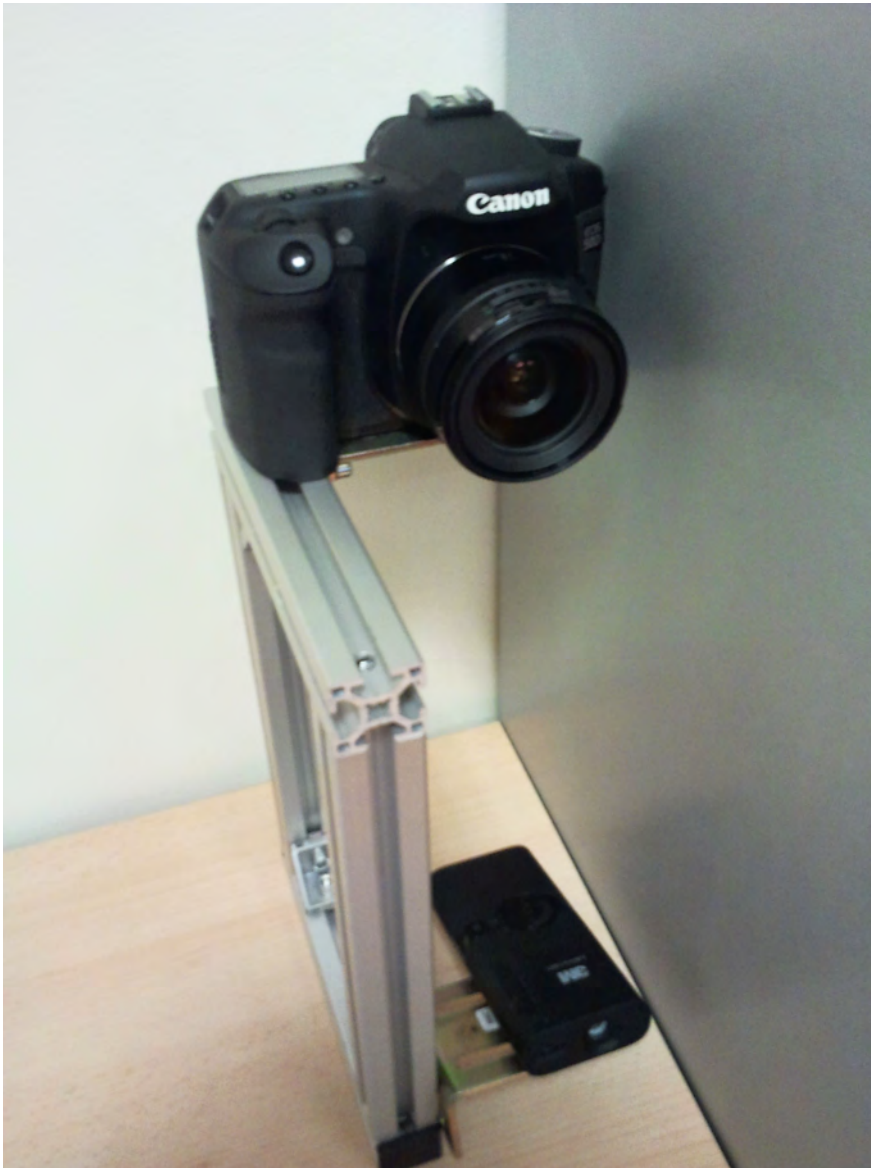
Figure 5.7: Proposed setup: a portable frame with the camera and the pico-projector attached on it.
