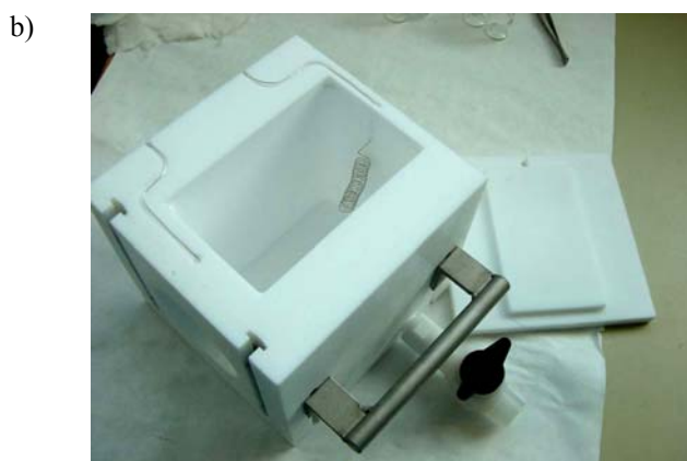
Fig. 5.2. The lateral-wafer cell used for the fabrication of porous silicon layers a) schematic of the cross sectional view. b) photograph of cell.
