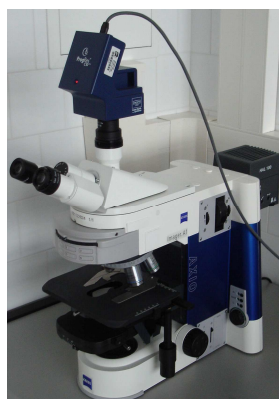
Figure 4.4: Optical microscope Carl Zeiss Axio Imager A1 with CCD camera ProgRes C10 from JenOptik.
