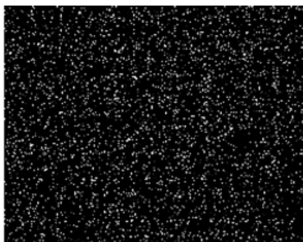
Figure 3. SEM-EDX Si-mapping of cross-section of ELO 5 wt.-% G-POSS nanocomposite.
