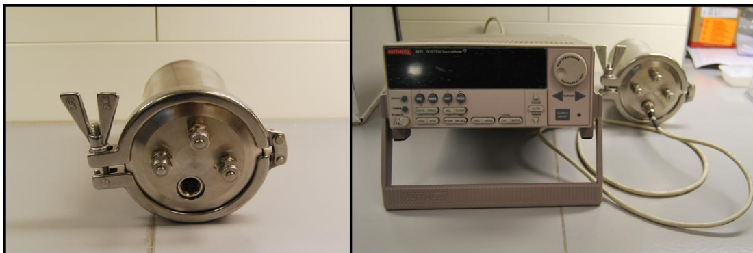
Figure 12. Image of the gas chamber (left) and the gas chamber connected to the Keithley 2611 System SourceMeter (right).
