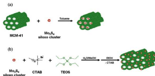
Scheme 2. A schematic representation of the preparation of the hybrid silica materials by using the grafting approach (a) and the in situ approach (co-condensation) (b).
