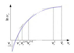
**Fig. 6.** Approximation of the  $\ln v_r$  function by *L* supporting hyper-planes.
