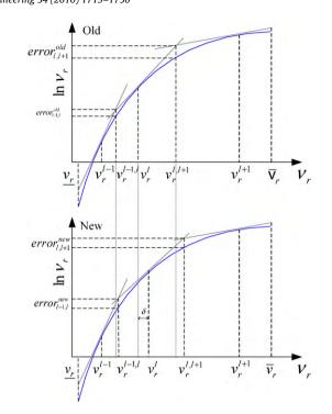
**Fig. 7.** Illustration of the decrease in *error*<sub>max</sub> by moving  $SH_l$  a distance  $\delta$  towards the vertex  $v_r^{l,l+1}$ .
