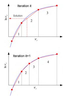
**Fig. 3.** Piecewise grid update example. As the solution of the first iteration is found in the second interval, it is split into two sub-intervals for the next iteration.
