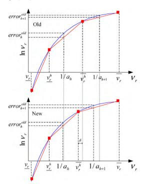
**Fig. 9.** Illustration of the decrease in *error*<sub>max</sub> by moving the grid point  $\overline{v_r^h}$  a distance  $\delta$
