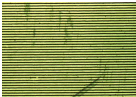
Fig. 1. Optical microscopy image of the diffraction grating generated on the surface of an RTP crystal by ultrafast laser ablation.
