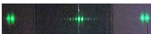
Figure 1.6. Nonlinear diffraction patterns generated in a 1D QPM grating in a periodically poled lithium niobate crystal [55].
